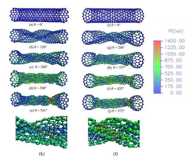
Fig. Snapshot of failure of (10, 10) and (0, 17) BNNTs under torsional deformation.
