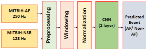
Figure 3: Proposed block diagram for detecting AF and non AF
