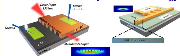
Optical modulator based on semiconductor heterojunctions: utilization of ENZ property of ITO
