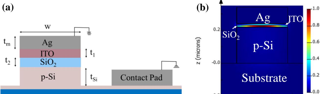
Fig. S3. (a) Cross-sectional view of the engineered multilevel nanophotonic resistive switch and (b) Corresponding mode profile distribution at the telecommunication wavelength of  $1.55 \mu\text{m}$ . Here, the thickness of the Ag, ITO,  $\text{SiO}_2$  and Si has been considered as respectively,  $t_m$ ,  $t_1$ ,  $t_2$ ,  $t_{\text{Si}}$ . The widths of the device is consider as  $w$ .
