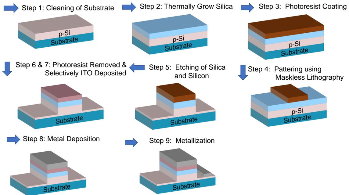
**Fig. S1.** 3D-schematic illustrates the standard CMOS-compatible fabrication process of the proposed engineered multilevel hybrid plasmonic waveguide on a p-type SOI wafer. The process involves sequential cleaning steps, thermal treatment of silica, photoresist coating, lithography patterning, wet etching of silicon and silica, removal of photoresist, deposition of ITO using RF sputtering, metal deposition via DC sputtering, and completion of metallization.
