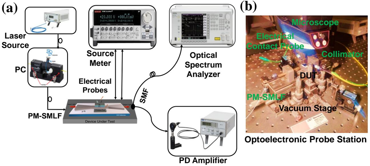
Fig. S2. Experimental optoelectronic characterization setup. (a) A schematic representation of setup comprising a laser source, polarization controller, tapered-lens PM SMF, optoelectronic probe station with the device under test (DUT), vacuum stage, microscope, source meter, OSA, and photodiode amplifier. The  $1.55 \mu\text{m}$  wavelength laser source has been used for read the multiple optical states. (b) Image of DUT on the optoelectronic probe station.
