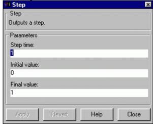
The default parameters in this dialog box generate a step function occurring at time=1 sec, from an initial level of zero to a level of 1. (in other words, a unit step at t=1). Each of these parameters can be changed. Close this dialog before continuing.
