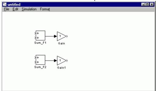
These Gain blocks should contain 1/M for each of the masses. We will be taking these variable as M1 and M2 from the MATLAB environment, so we can just enter the variable in the Gain blocks. Double-click on the upper Gain block and enter the following into the Gain field.
