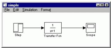
The *simple* model (from the <u>model file</u> section) consists of three blocks: Step, Transfer Fcn, and Scope. The Step is a **source block** from which a step input signal originates. This signal is transferred through the **line** in the direction indicated by the arrow to the Transfer Function **linear block**. The Transfer Function modifies its input signal and outputs a new signal on a line to the Scope. The Scope is a **sink block** used to display a signal much like an oscilloscope.
