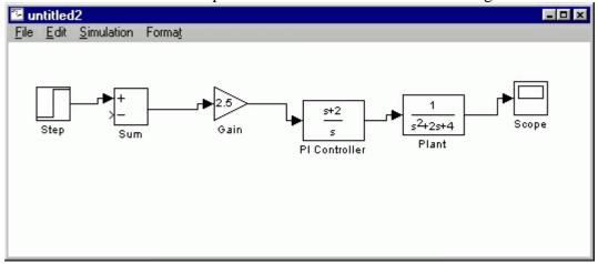
• The line remaining to be drawn is the feedback signal connecting the output of the Plant to the negative input of the Sum block. This line is different in two ways. First, since this line loops around and does not simply follow the shortest (right-angled) route so it needs to be drawn in several stages. Second, there is no output terminal to start from, so the line has to tap off of an existing line.
