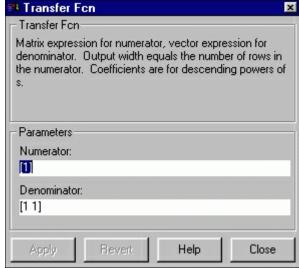
This dialog box contains fields for the numerator and the denominator of the block's transfer function. By entering a vector containing the coefficients of the desired numerator or denominator polynomial, the desired transfer function can be entered. For example, to change the denominator to  $s^2+2s+4$ , enter the following into the denominator field:
