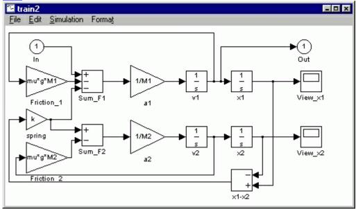
Save this model as **train2.mdl** or download our version <u>here</u>. Now, we can extract the model into MATLAB. Enter the following command at the MATLAB command window to extract a state-space model.
