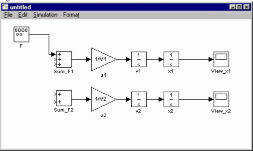
The next force acting on M1 is the friction force. This force is equal to:  $F_fiction_1=mu*g*M1*v1$
