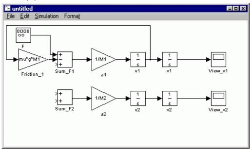
The last force acting on M1 is the spring force between masses. This is equal to: k\*(x1-x2)
