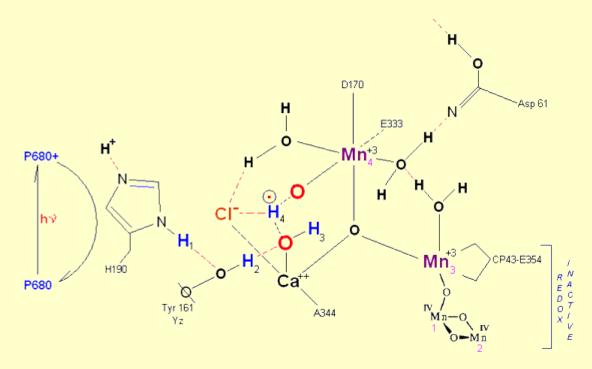
**State S1':** P680+ is reduced by Yz. Hydrogen bridge forms as in So  $\rightarrow$ S1, charged stabilized by Cl-. Note that both hydrogens on the reactive Water molecule number 1 has transferred to reactive water molecule number 2 via a hydronium radical bridge transfer mechanism.
