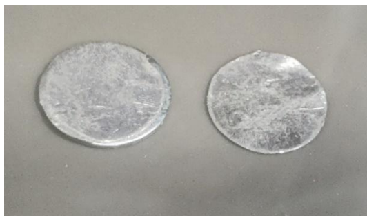
Figure S6 Images of Li metal before (right) and after (left) contact with PE20.
